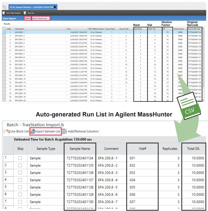
In this example, the original barcode from the unprepared sample was used as the sample name in MassHunter's run list, alongside dilution factors and the sample preparation procedure allowing for easy tracking in the LIMS system.
